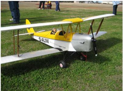
The Moth is from the Flair kit with operating "doors", proper flat flying wires and the corrugations on the wing tank made from plastic material used on model railway buildings - oh and a sprung u/c too.
